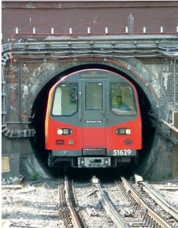
The nickname "Tube" comes from the circular tube-like tunnels through which the small profile trains travel.
